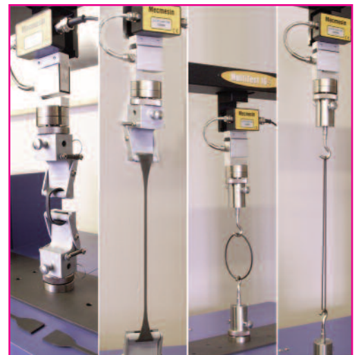
Spring Loaded Fold Grips and Test Hooks used to test different samples
