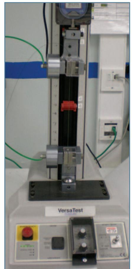
VersaTest system shown with BFG testing guidewire
